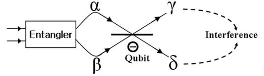
**Figure 2.** A schematic diagram of a charge qubit and a detector that injects spin-entangled electrons.
