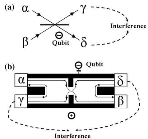
**Figure 1.** (a) A schematic diagram of a charge qubit electrostatically coupled to a detector composed of a beam collider and four (two input and two output) electrodes, (b), which can be realized, for instance, by using the quantum Hall bar and quantum point contact.
